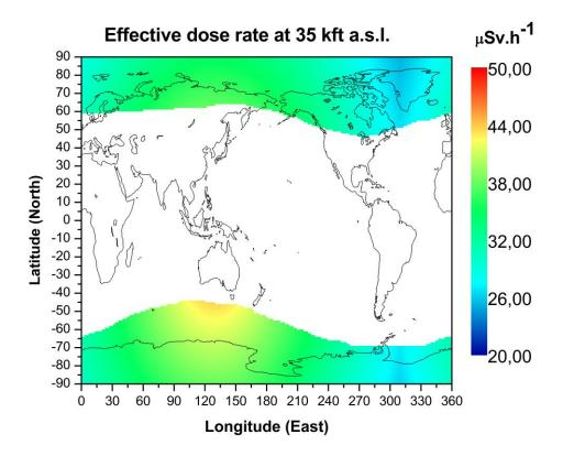
Map of radiation dose at 35 kft altitude in the polar region (color scale on the right, cf. the average recommended upper dose for public which is ~0.11  $\mu$ Sv/h) during the solar particle storm of 13 December, 2006, which is 30-50  $\mu$ Sv (corresponding to a 2-3-week normal dose) during one hour. During severe events, the annual recommended dose can be reached or even exceeded during one flight. (Adopted from Mishev & Usoskin, JSWSC, 5, A10, 2015).
